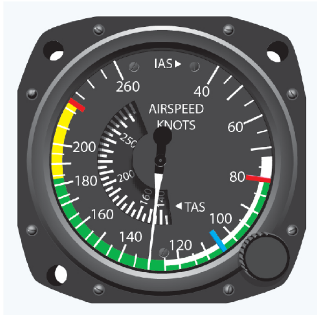
Figure 13-1. Airspeed indicator markings for a multiengine airplane. Source: FAA Airplane Flying Handbook (FAA-H-8083-3C), Ch. 13.
